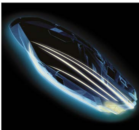
Hard-chine planing hull with variable deadrise (Flybridge and Atlantis Collections)
