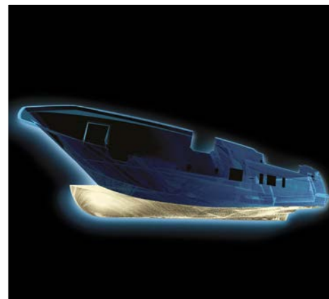
D2P (Displacement to Planing) hull with a double chine and wave piercer (reserved for several models in the Grande Collection)
